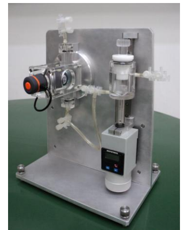
Right: micromanometer, specially designed for small pressure differential measurements in the riblets section.
