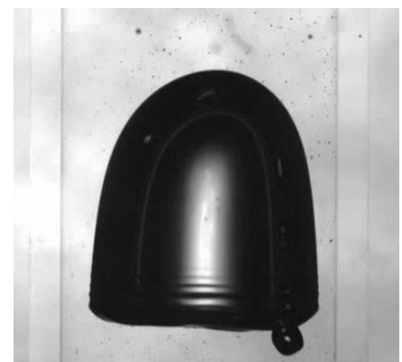
Visualization of a Taylor bubble with the pulsed shadow (PST) technique.
