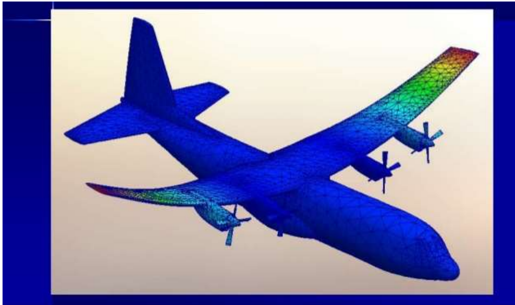
Extraído de C-130 cargo aircraft vibration mode shapes in flight Don Blanchet 3B Associates
