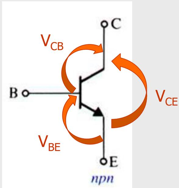
$$V_{CE} = V_{CB} + V_{BE}$$
